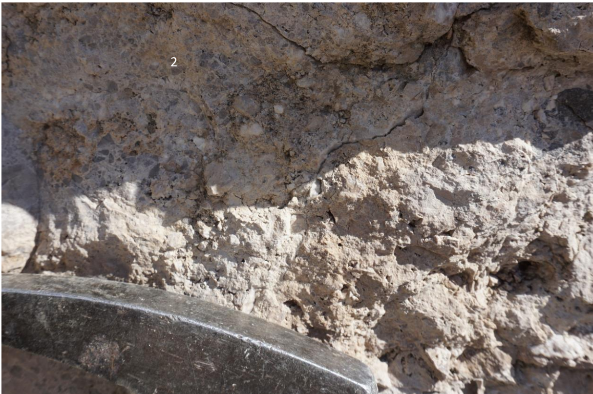
2: The smooth slickenside surface was formed on a tectonic breccia (i.e. cataclasite). Cataclasites are found where high shear strain causes fracturing at the contact of two rock surfaces, such as at fault and thrust planes.
