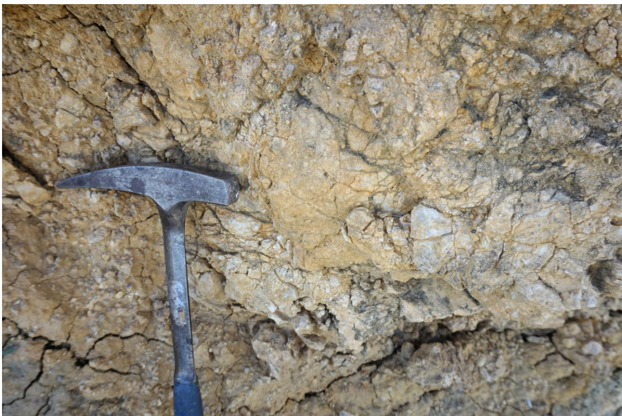
1: Highly sheared Pindos limestone at base of nappe and contact to flysch.
